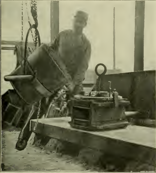
Fig. 6—Pouring Driving Box Crown Brass and Hub Liner.
